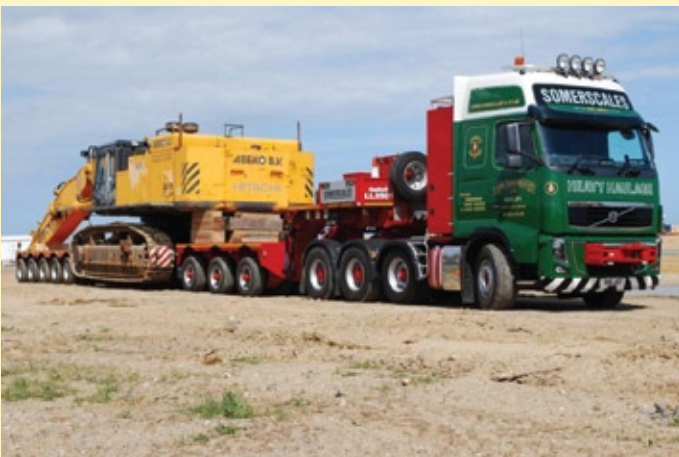
100t excavator transported from Great Yarmouth to Immingham.
